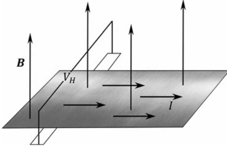
Figure 4: The shaded region represents the slab-like conductor or semiconductor, with  $I$  the current passing through it,  $B$  the magnetic field perpendicular to it, and  $V_H$  the Hall voltage measured transverse to the current.
